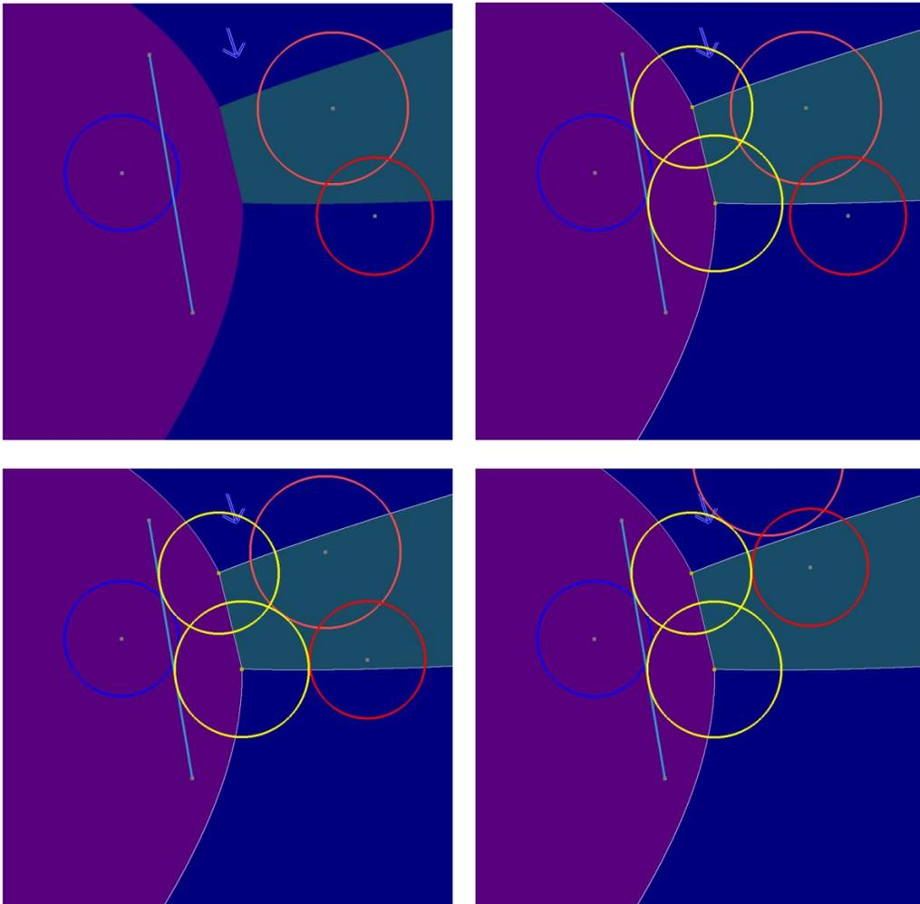
Fig. 2:  $L(CL, CC)$  example. *Top left*: Fixed cluster in blue, moving cluster in red, arrow shows translation direction. *Top right*: Two solution found by intersecting the cyclographic maps of the fixed-cluster objects with the purple surface obtained by sweeping the conic intersection of the two cyclographic maps of the moving cluster circles. *Bottom*: the two solutions with the moving cluster translated as required.
