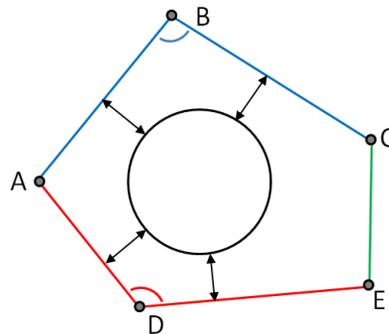
Fig. 1: Rotational cluster merge with a variable-radius circle from four constraints: Lengths  $(A,B)$ ,  $(B,C)$ ,  $(A,D)$ , and  $(D,E)$  and angles  $(A,B,C)$  and  $(E,D,A)$  are given. The circle is to have a prescribed distance from the blue and the red sides. No symmetry is required.
